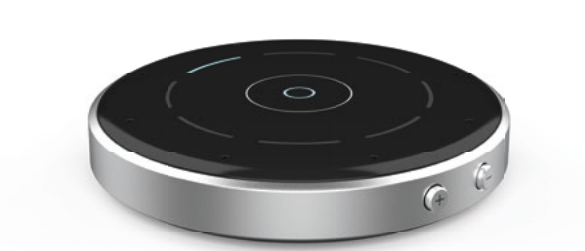
Figure 1. Table Microphone in Automatic Mode. The active direction of the beamformer is shown by the illuminated segment.
