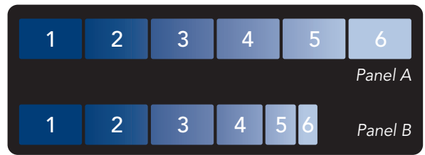
Figure 3. In this illustration, the numbered boxes represent hearing aid channels; the increasing channel number represents increasing frequency. Panel A shows the conventional hearing aid processing and Panel B shows the compressed information and its relationship to the lower frequency information.
